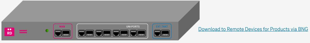
Each UNI allows port-based or VLAN-based configuration, with the respective possible number of EVCs
